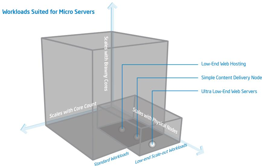
**Figure 2.** This 3D diagram shows that ideal workloads for micro servers are those that tend to have relatively lower processing requirements and scale best by adding more interconnected physical nodes.
